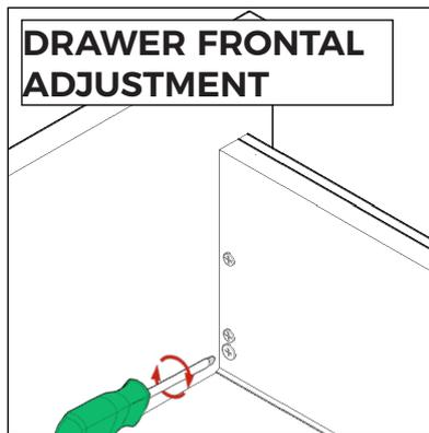
Loosen top 2 screws. Turn bottom screw to adjust drawer frontal height, once in desired position re-tighten the top 2 screws.
