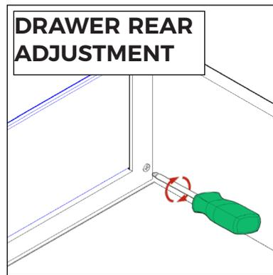
Turn screw to adjust rear elevation of drawer.
