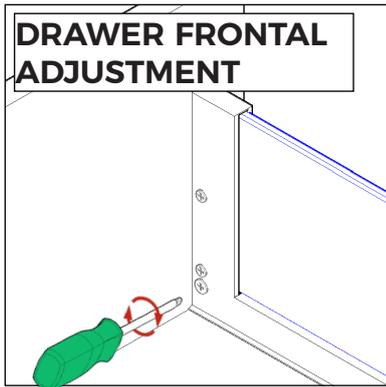
Loosen top 2 screws. Turn bottom screw to adjust drawer frontal height, once in desired position re-tighten the top screws.
