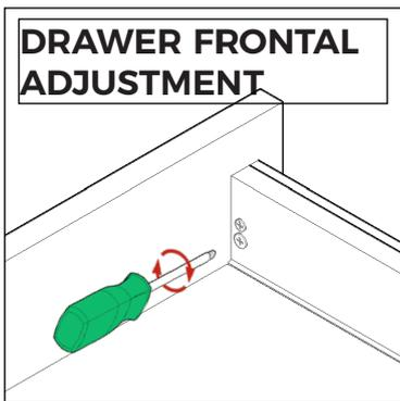
Loosen top screw. Turn bottom screw to adjust drawer frontal height, once in desired position re-tighten the top screw.
