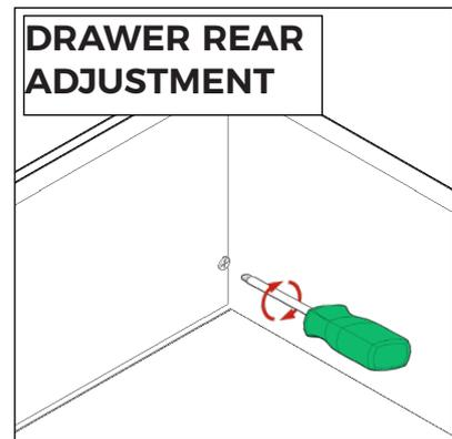
Turn screw to adjust rear elevation of drawer.
